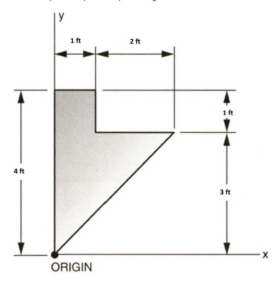
Find the centroid of the shape with respect to the point of origin shown.
